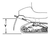
To set up the EDGE RMK rear suspension torsion spring preload, measure the distance between the ground and rear bumper (see illustration). This measurement should be taken with no rider and the rear suspension at full extension. This is measurement X.
